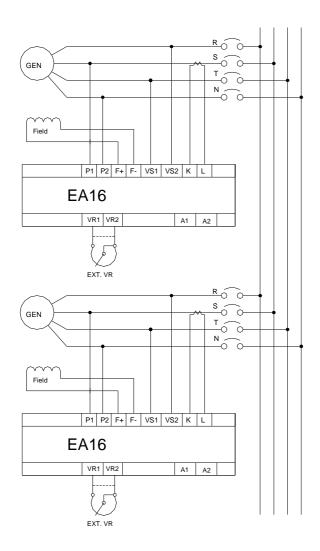
Figure 2 Paralleling Connection
